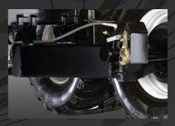
Stability is greatly improved with the Javlor-designed walking beam due to the wide tire track and lower center of gravity, critical when dumping materia in soft and uneven terrain. Commercial grade axles are cambered\* for better tire life and balanced all-wheel ground contact.
